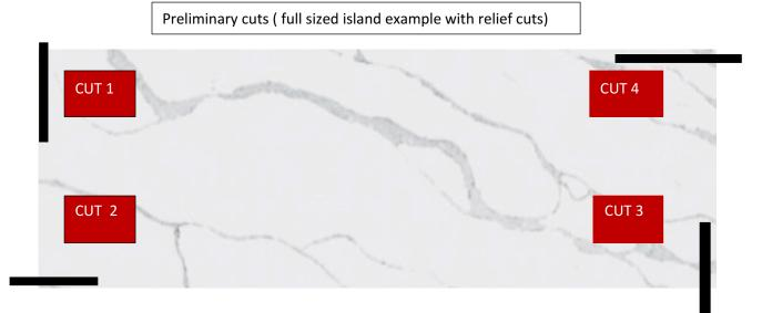
Common straight line cutting procedure CUT 2 CUT 1 12"-20" Preliminary relief cuts (1 per quadrant)
